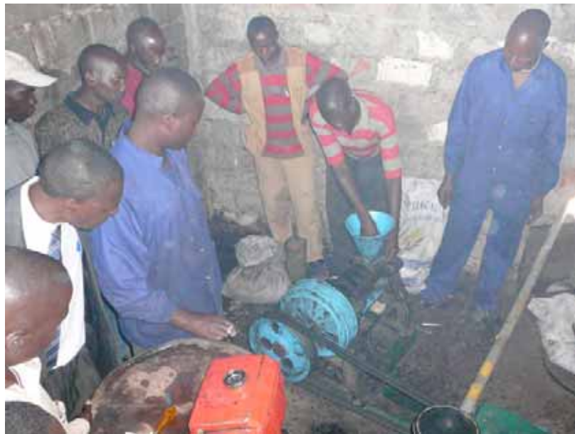
Demonstrating the pressing of oil from sunflower seeds on a press powered by the 2-cylinder Lister engine run on cottonseed oil in the dual fuel system.
